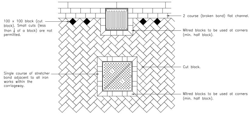
In block paved areas all ironwork shall be 150 deep to allow blocks to be laid up to the frame of gully gratings and manhole covers.
