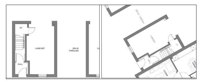
Having the side door opening outwards significantly compromises the usable space for parking to only 1.7m wide, rendering the use unattractive. To address this issue, the side doors need to be designed to open inwards rather than outwards.
