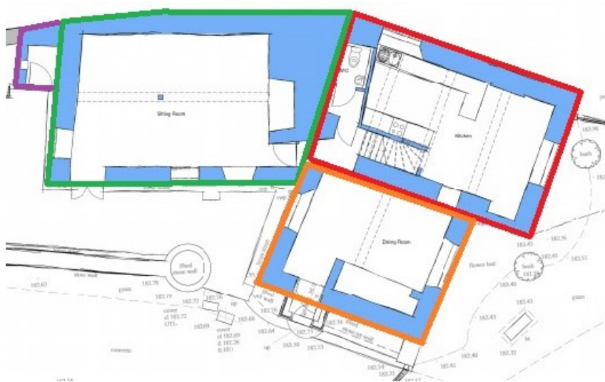
Ground floor plan showing the sequence of construction. (17 th century red; late 18 th /early 19 th century green; later 19 th century orange; 20 th century purple).
