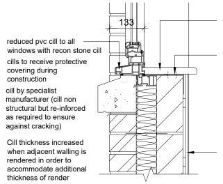
cill to be recon stone or concrete (painted on insitu with external quality masonry paint). If cill does not comply with manual handling limits then suitable lifting eyes are to be incorporated.
