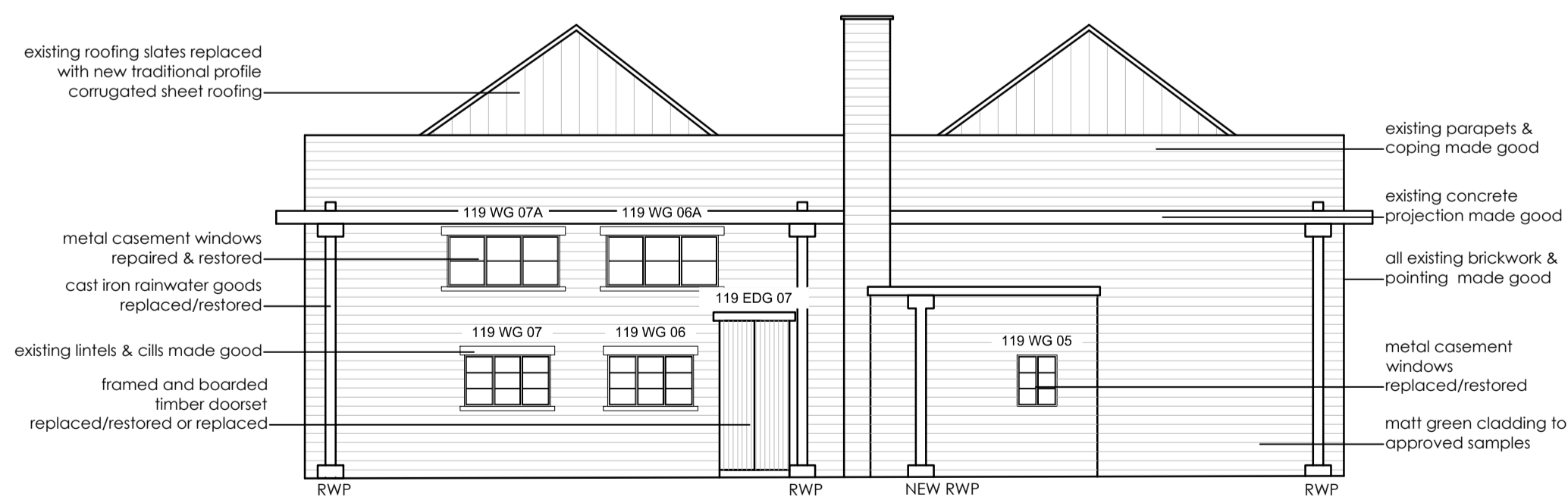
BUILDING 119 SOUTH ELEVATION - PROPOSED
