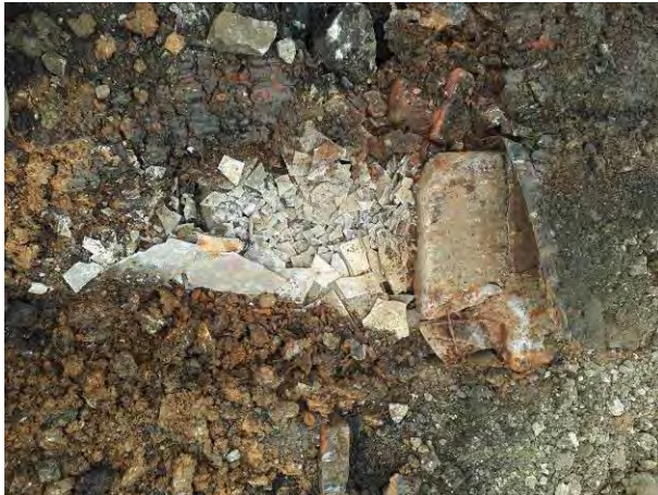
20.06.18 – Cache of broken fragments of ACM cement sheeting discovered within contamination hotspot.
