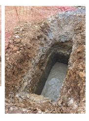
The results of the soakage testing are enclosed and the table overleaf provides a summary of the results of testing at each of the locations indicated on the site plan that was provided by the Civil Engineers and set out on site by the Ground Workers. The trial pits were excavated using a mechanical excavator with breaker and ripper that was provided by the Ground Workers.
