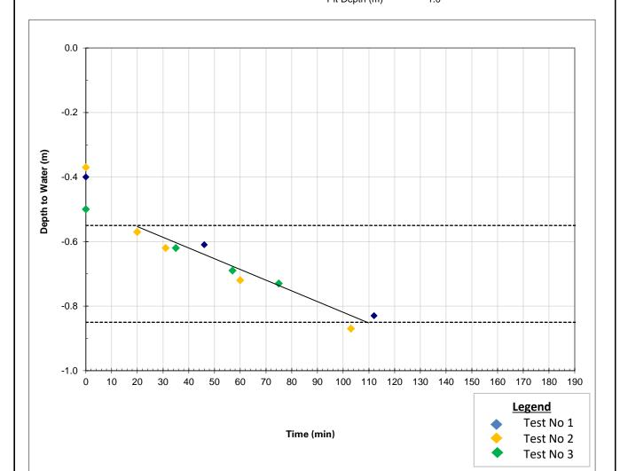
Design Soakage Rate 2.3E-05 m/s (based on linear portion of graph as shown) 1.98 m/day
