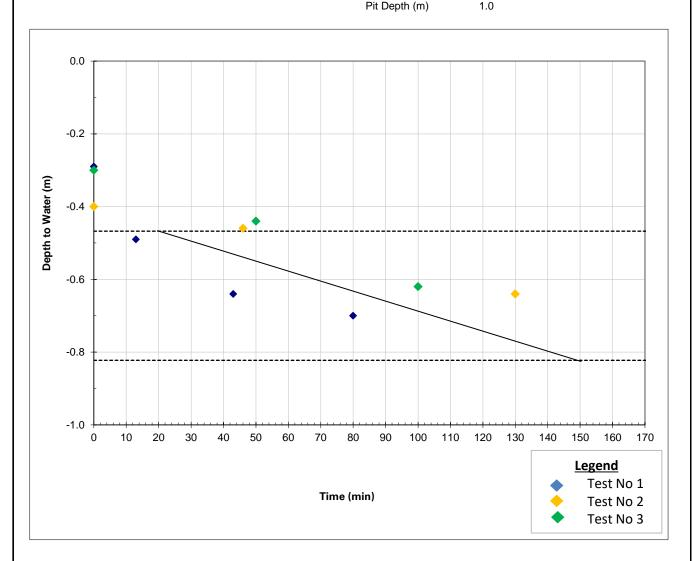
Design Soakage Rate 1.7E-05 m/s (based on linear portion of graph as shown) 1.44 m/day
