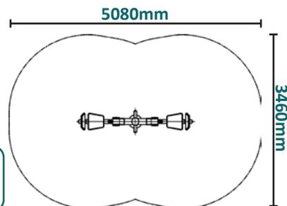
Unit Weight : 84kg Unit Free Fall Height : 1060mm
