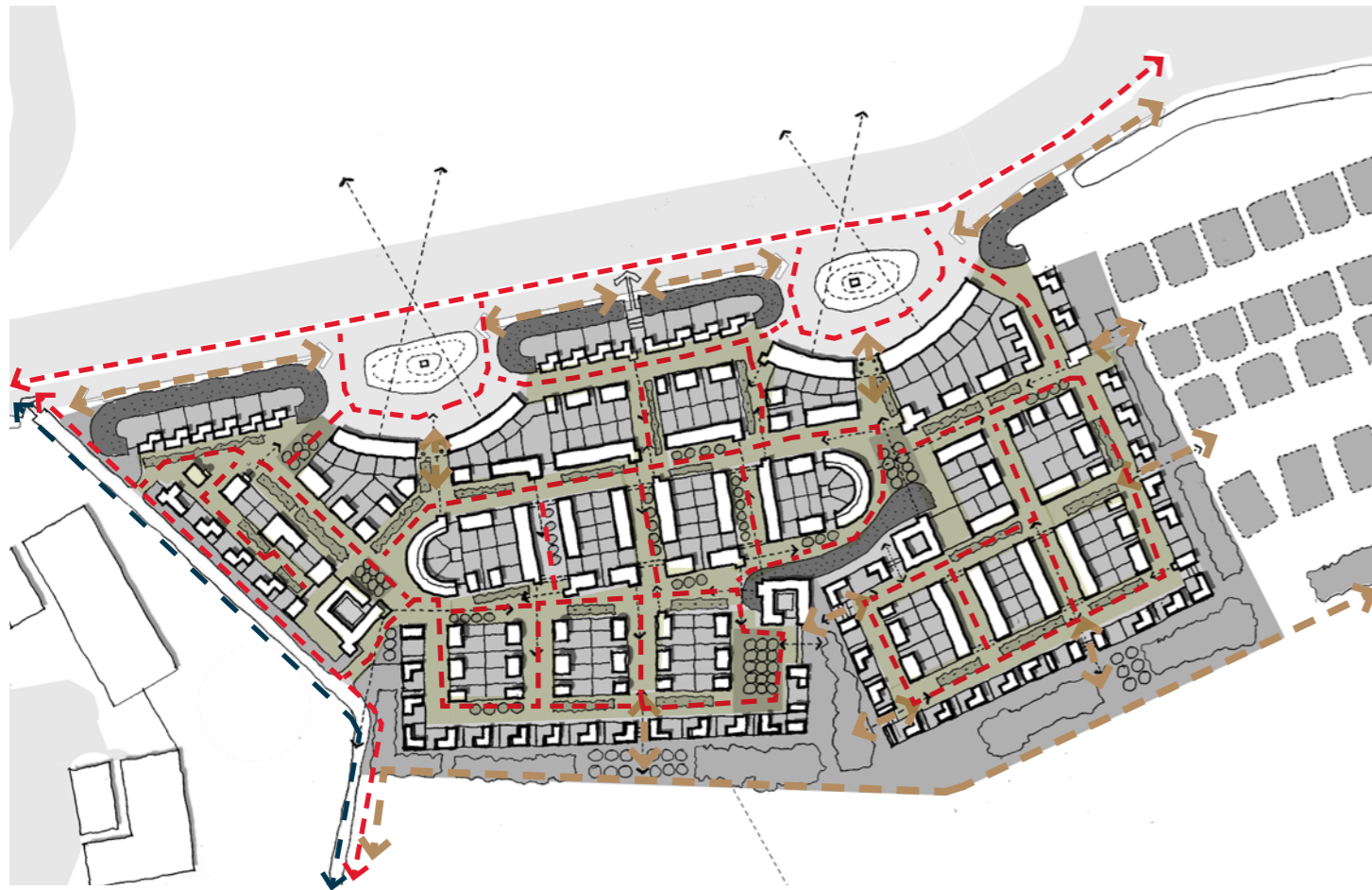
Movement & Access - A permeable and walkable urban quarter with pedestrian priority shared surface streets that harbour places for social interaction and community cohesion.
