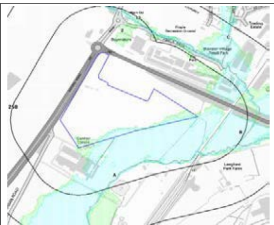
Figure 3-4 Extract of GroundSure report showing extent of flooding modelled from the Lanford Brook
