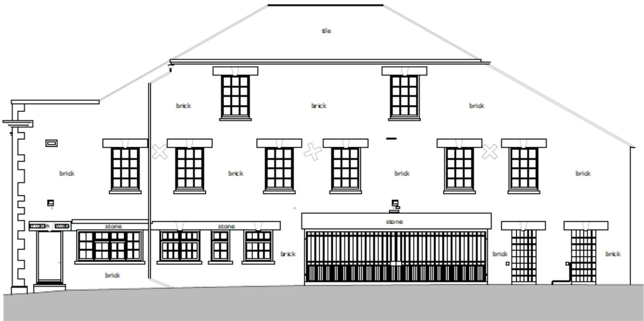
Figure 10.0 – Existing west elevation
