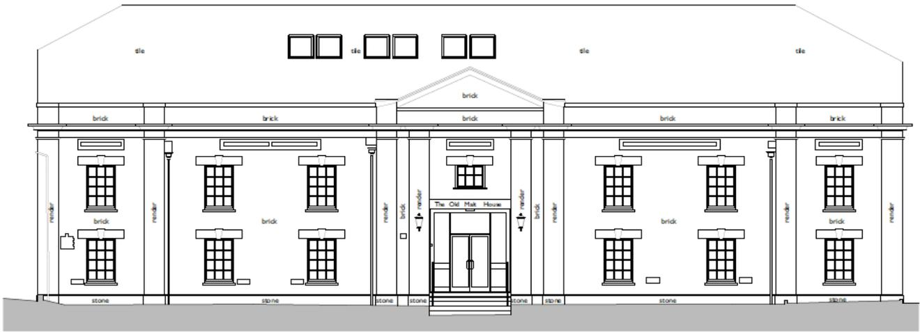
Figure 12.0 – Existing north elevation
