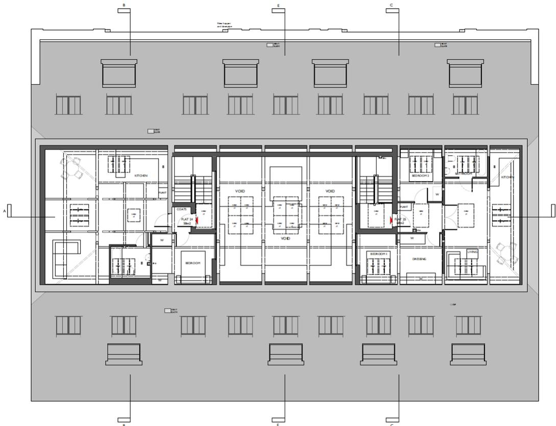
**Figure 33.0** – Proposed third floor plan
