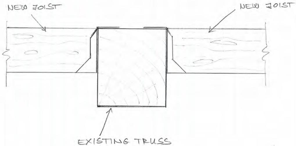
D03 TIMBER FLOOR JOIST DETAIL
