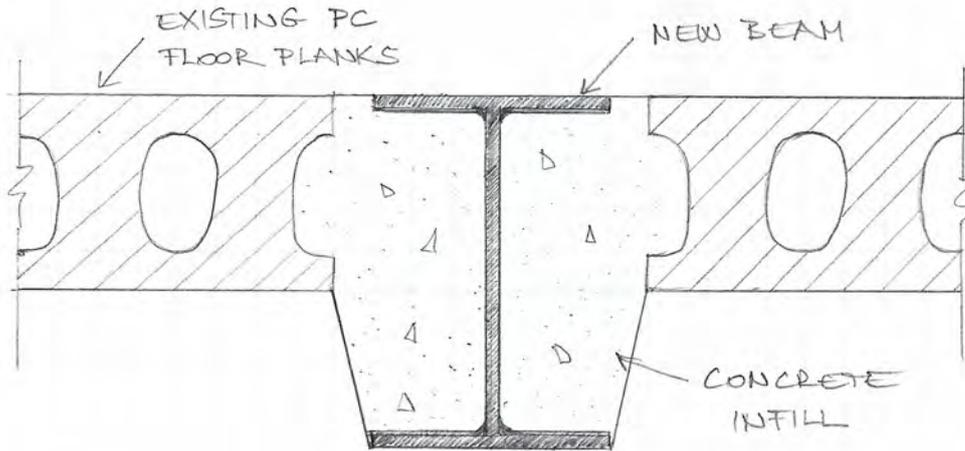
D05 NEW BEAM IN EXISTING UNIT FLOOR
