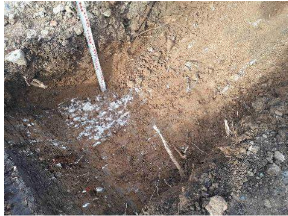
06.11.18 – TP5 Soil profile - weathered bedrock at base
