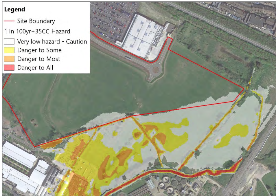
Figure 4.4 Flood hazard map for the 1 in 100 year including 35% allowance for climate change
