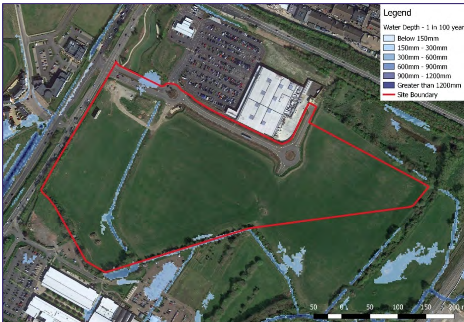
Figure 4-5 EA's surface water flood depth map for 1 in 100 annual probability event with indicative red line boundary. Accessed 16/8/17 (© Environment Agency copyright and/or database right 2015. All rights reserved. Some features of this map are based on digital spatial data from the Centre for Ecology & Hydrology, © NERC (CEH) and © Lead Local Flood Authorities. Soils Data © Cranfield University (NSRI) and for the Controller of HMSO 2013. Imagery © Google 2017, Map data © Google 2017)
