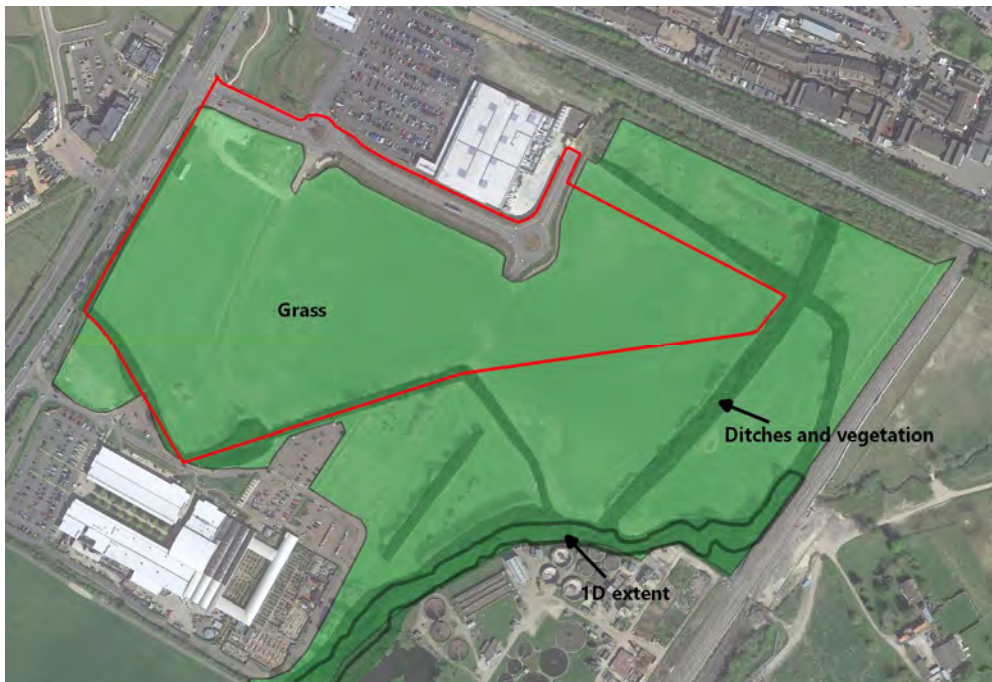
Figure 2.5 Illustration of the extent that different Manning’s roughness values were applied in the 2D component of the BuroHappold BOP 2018 model.
