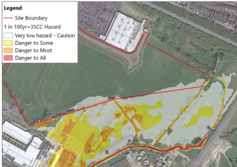
Figure 4-3 Fluvial flooding hazard map for 1 in 100 year storm event + 35% climate change (Contains Environment Agency Information © Environment Agency and/or database right) Imagery © Google 2017, Map data © Google 2017)
