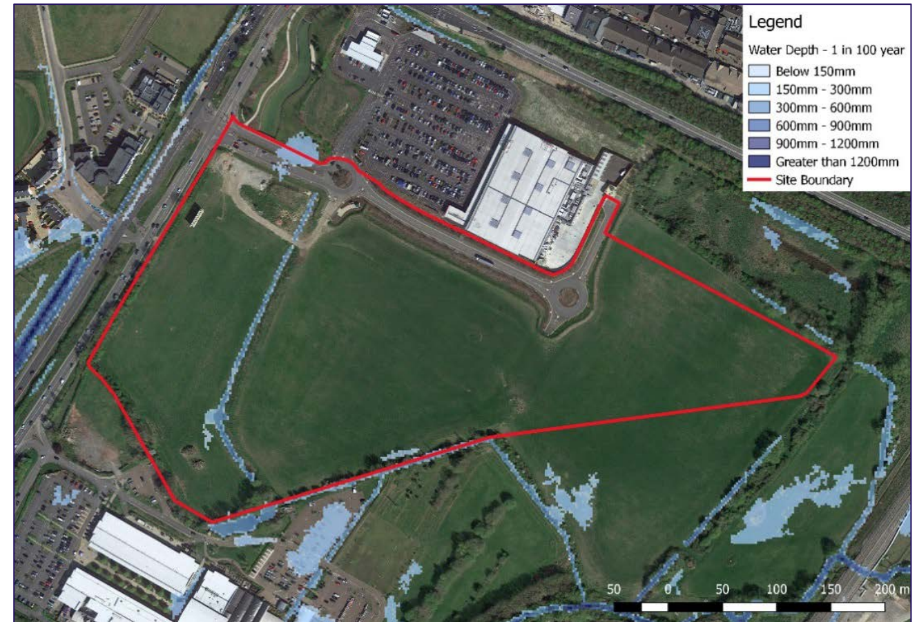
Figure 13.5 Environment Agency's surface water flood depth map for 1 in 100 annual probability event (© Environment Agency copyright and/or database right 2015. All rights reserved. Some features of this map are based on digital spatial data from the Centre for Ecology & Hydrology, © NERC (CEH) and © Lead Local Flood Authorities. Soils Data © Cranfield University (NSRI) and for the Controller of HMSO 2013. Imagery © Google 2017, Map data © Google 2017)
