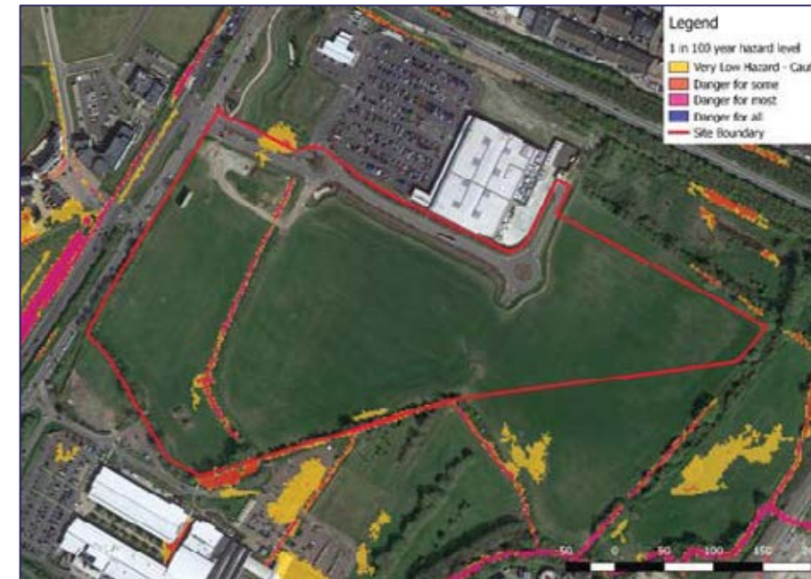
Figure 4-6 Environment Agency's surface water flood hazard map for the 1 in 100 annual probability event with indicative red line boundary. Accessed 16/8/17 (© Environment Agency copyright and/or database right 2015. All rights reserved. Some features of this map are based on digital spatial data from the Centre for Ecology & Hydrology, © NERC (CEH). Soils Data © Cranfield University (NSRI) and for the Controller of HMSO 2013. Imagery © Google 2017, Map data © Google 2017)
