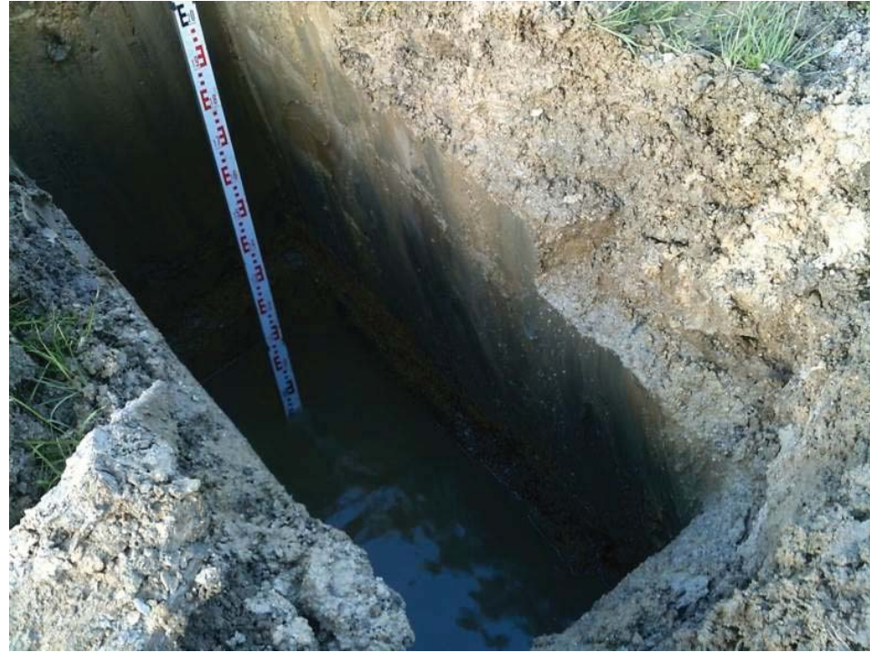
Trial pit 10 east face
