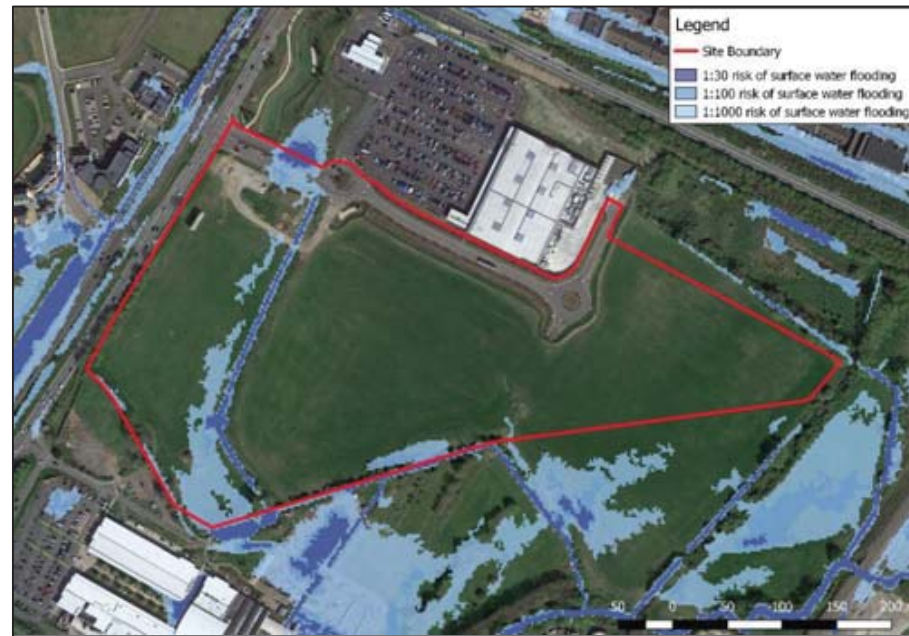
Figure 4-4 Environment Agency's surface water flood extents map with indicative red line boundary. Accessed 16/8/17 (© Environment Agency copyright and/or database right 2015. All rights reserved. Some features of this map are based on digital spatial data from the Centre for Ecology & Hydrology, © NERC (CEH). Soils Data © Cranfield University (NSRI) and for the Controller of HMSO 2013. Imagery © Google 2017, Map data © Google 2017)
