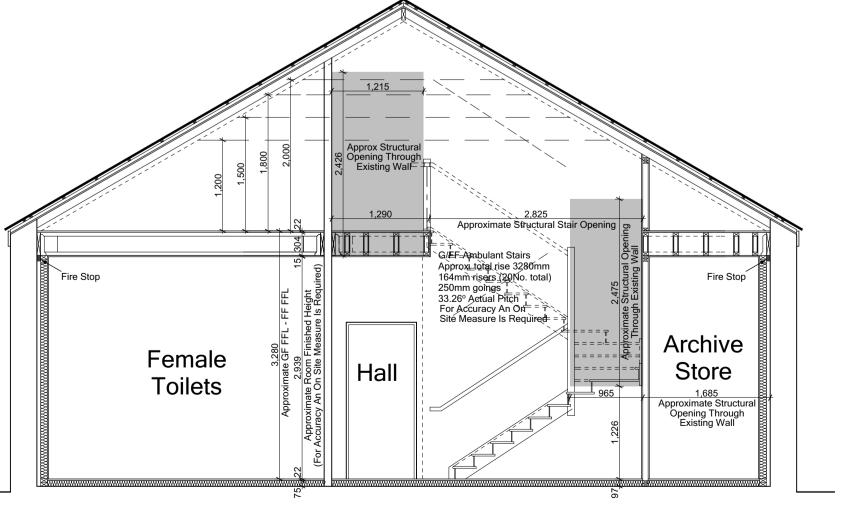
Existing door opening bricked up & made good New structural door opening to be created Section Through Stairwell Section Through Exhibition Hall
