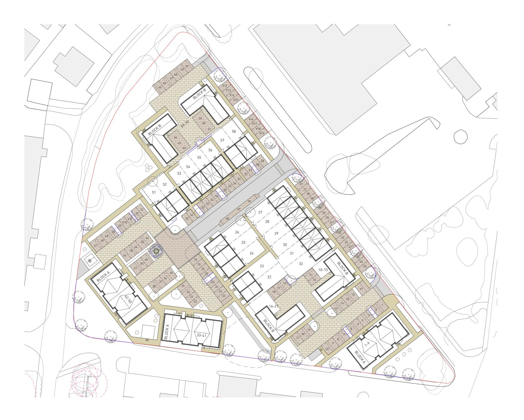
Existing vegetation to be retained to BS 5837 Front and rear footpaths, to be textured concrete paving flags laid in stack bond. E.g. Marshalls conservation texture flag paving in harvest buff or similar approved Tegular block paving or similar approved Contrasting tegular block paving to parking bays or similar approved Tegular setts Ornamental gravel- to be 20-30mm dia and laid over a semi-permeable weed suppressant Tree Root Barrier (eg ReRoot2000 by Green Blue
