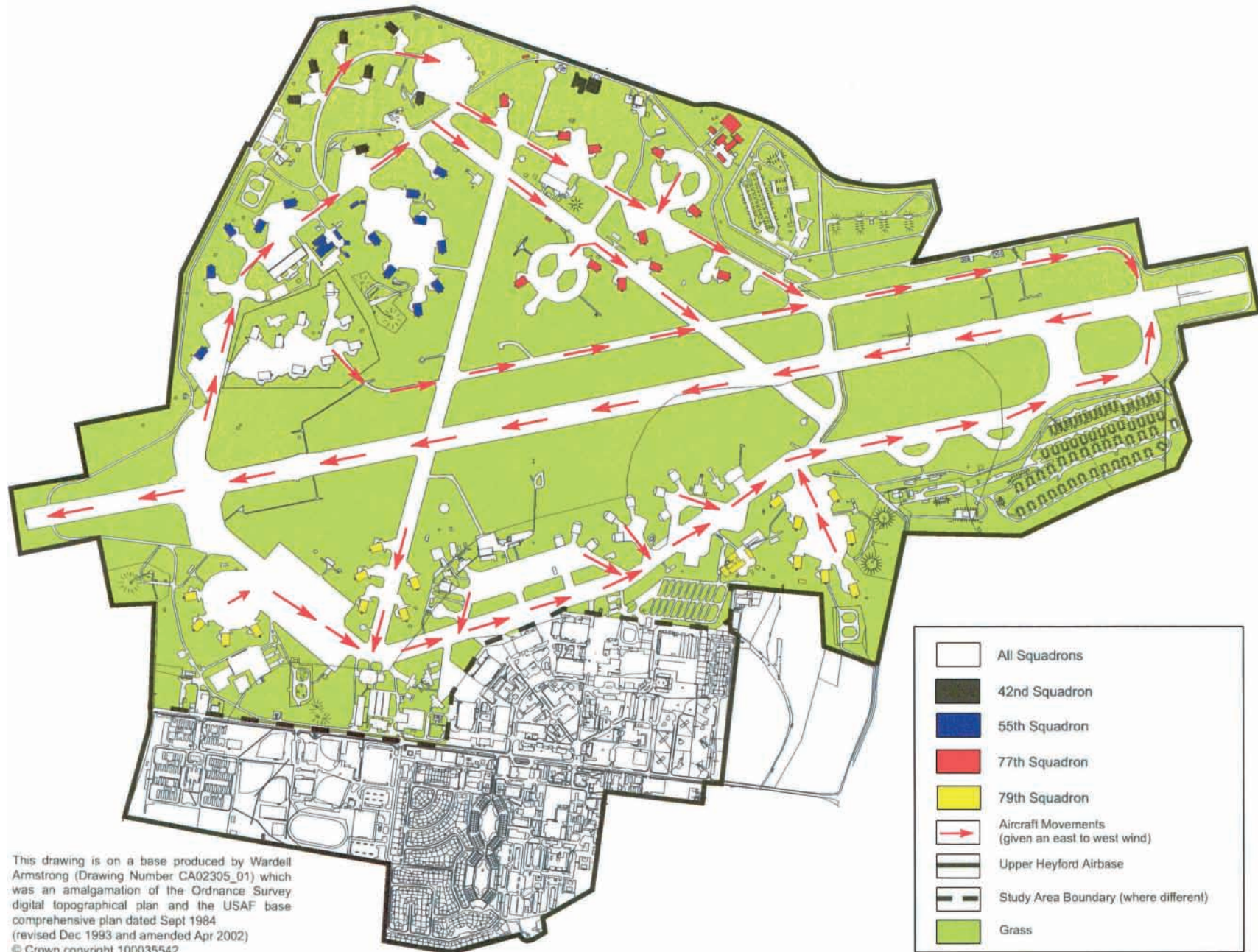
Figure 14: Grouping of the squadrons including the movement of aircraft along the taxiways prior to take off.
