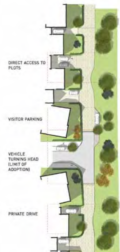
TYPICAL INDICATIVE PLAN SECTION LANES (GREEN EDGE) ST.5
