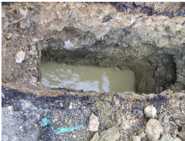
Photo 19 (left) showing trial pit 229, with Made Ground horizon
