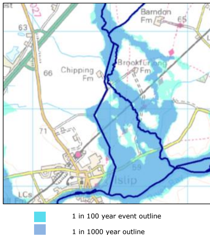
Figure 3 – Extract from the Environment Agency flood map (available online) showing extensive flood extent in the area.
