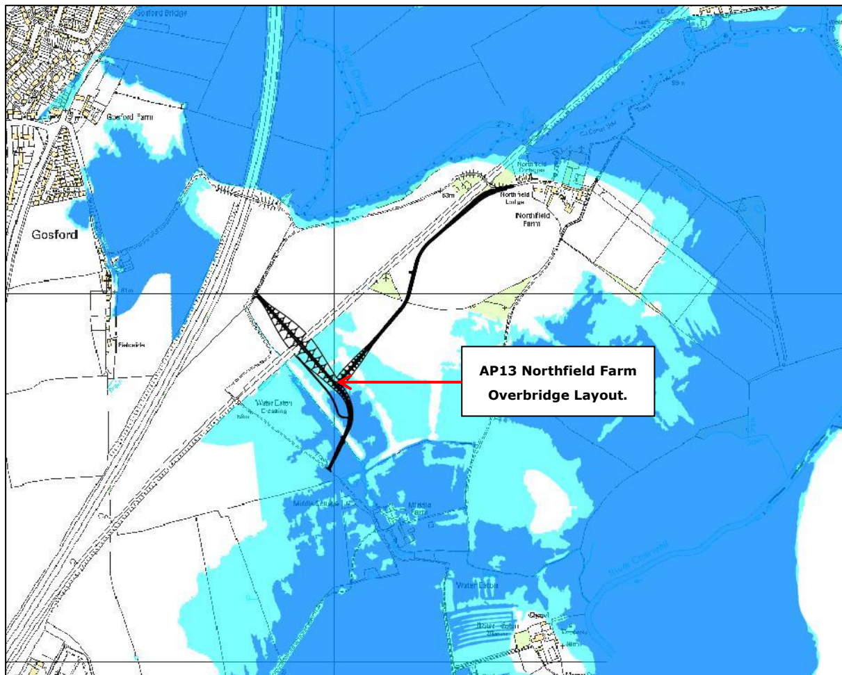
Figure 3 – Design Layout of the Proposed Northfield Farm Overbridge and Access Road (Provided by Atkins).
