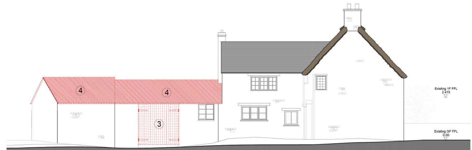
Existing Demolition Side Elevation
