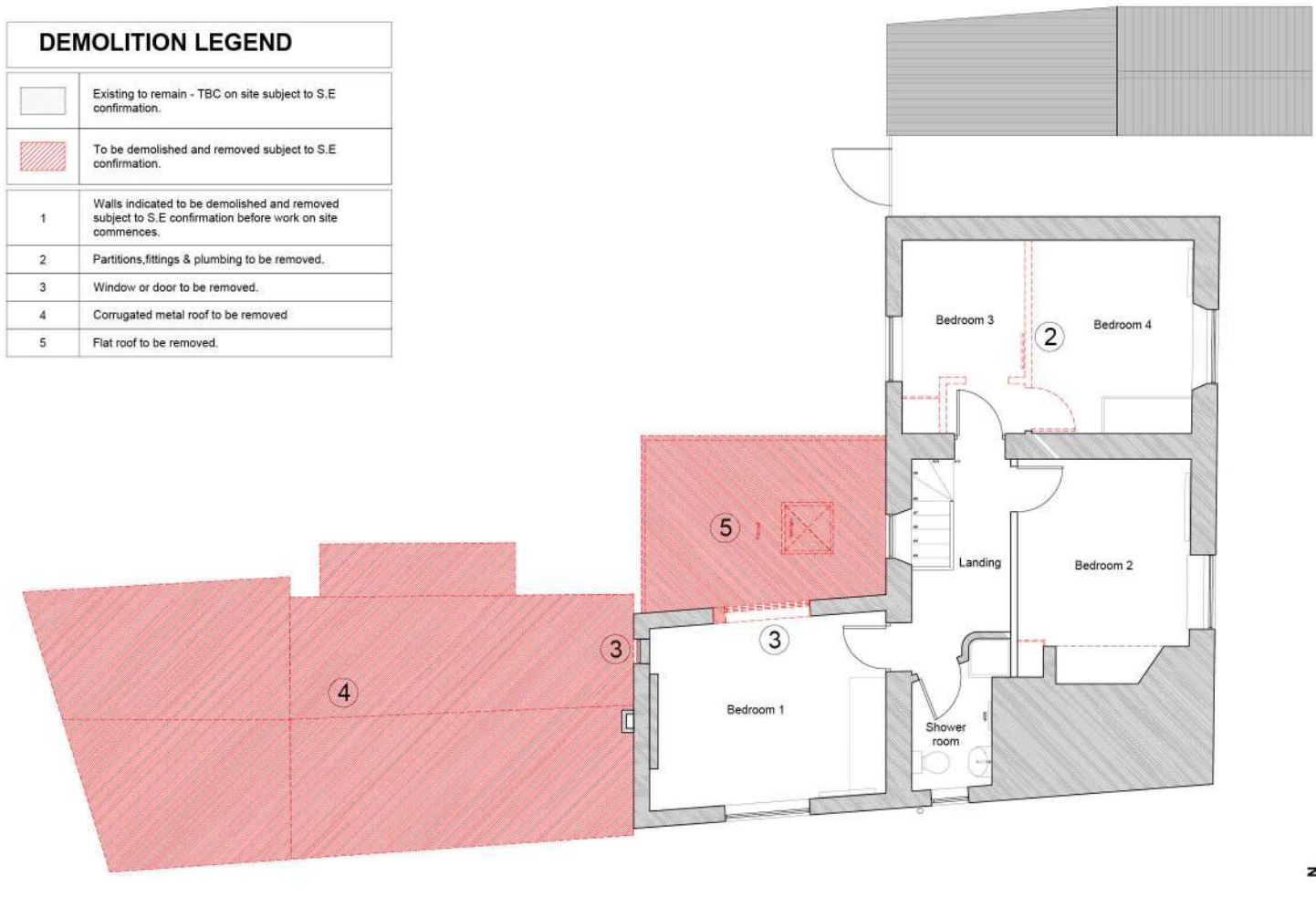
Existing Demolition First Floor Plan
