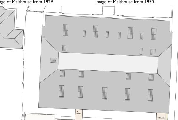
Image 18 Roof Plan showing proposed rooflights
