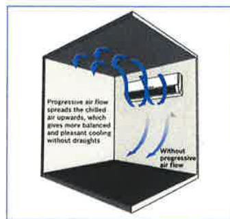
Cool air distribution in cooling mode
