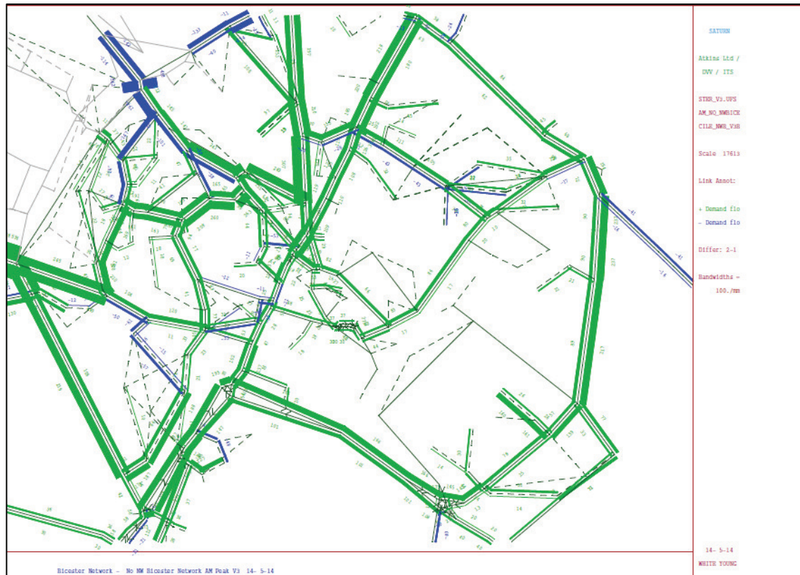
Figure 11-2: Difference in Traffic Flow of full NW Bicester Development over Reference Case 2031, AM Peak
