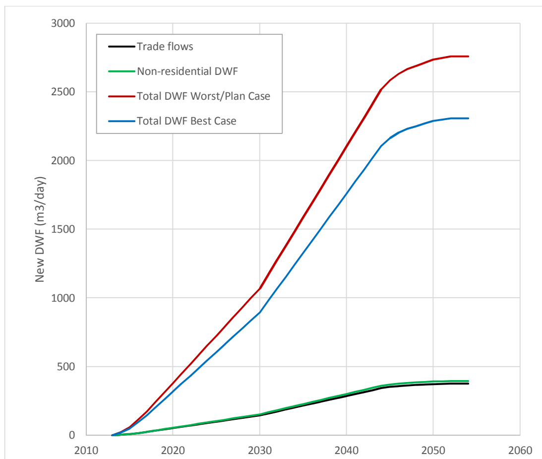
Figure 6-11 New DWF from NW Bicester development site
