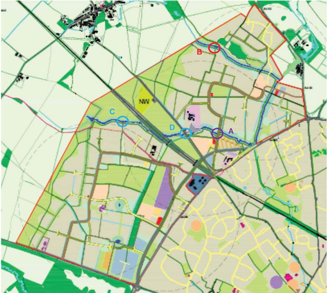
Figure 5-1 Proposed Watercourse Crossings (Primary road ringed in purple, secondary road ringed in red, existing crossings ringed in blue)
