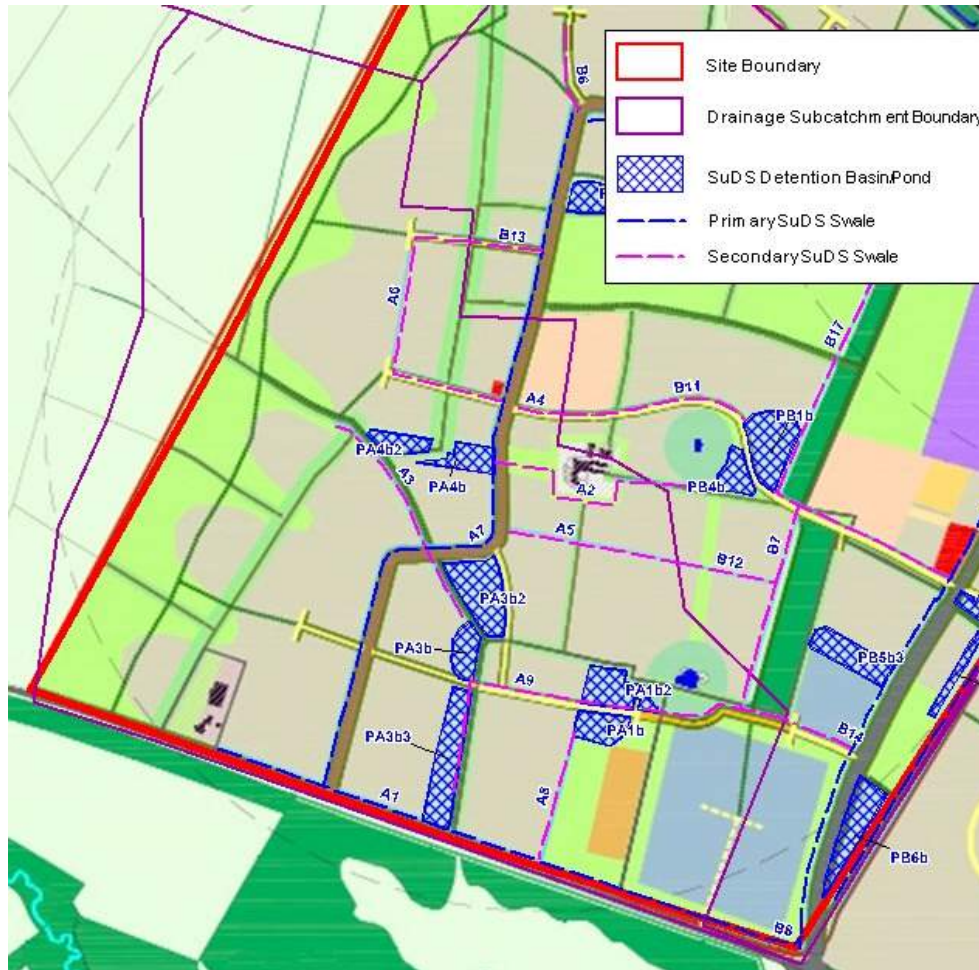
Figure 4-2 Drainage Catchment A SuDS Features
