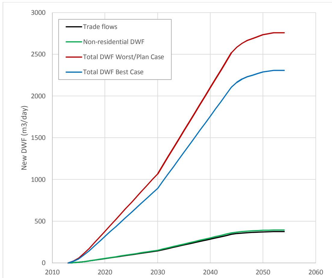
Figure 6-11 New DWF from NW Bicester development site
