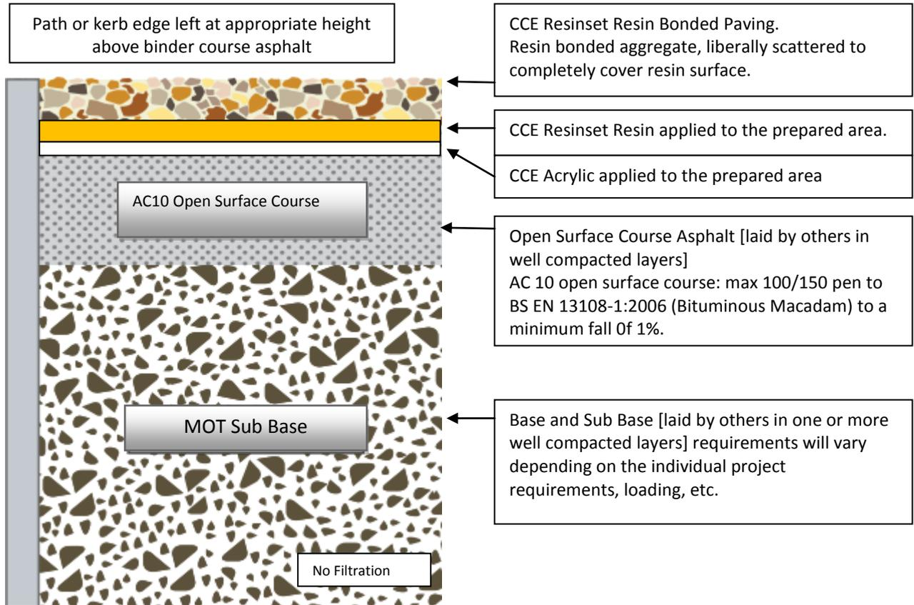
CCE Resinset bonded surfacing can be overlaid onto existing Asphalt or Concrete sub-bases, of suitable construction for the traffic expected. Cracks should be enlarged if necessary and filled with a Polymer/Cement filling material.
