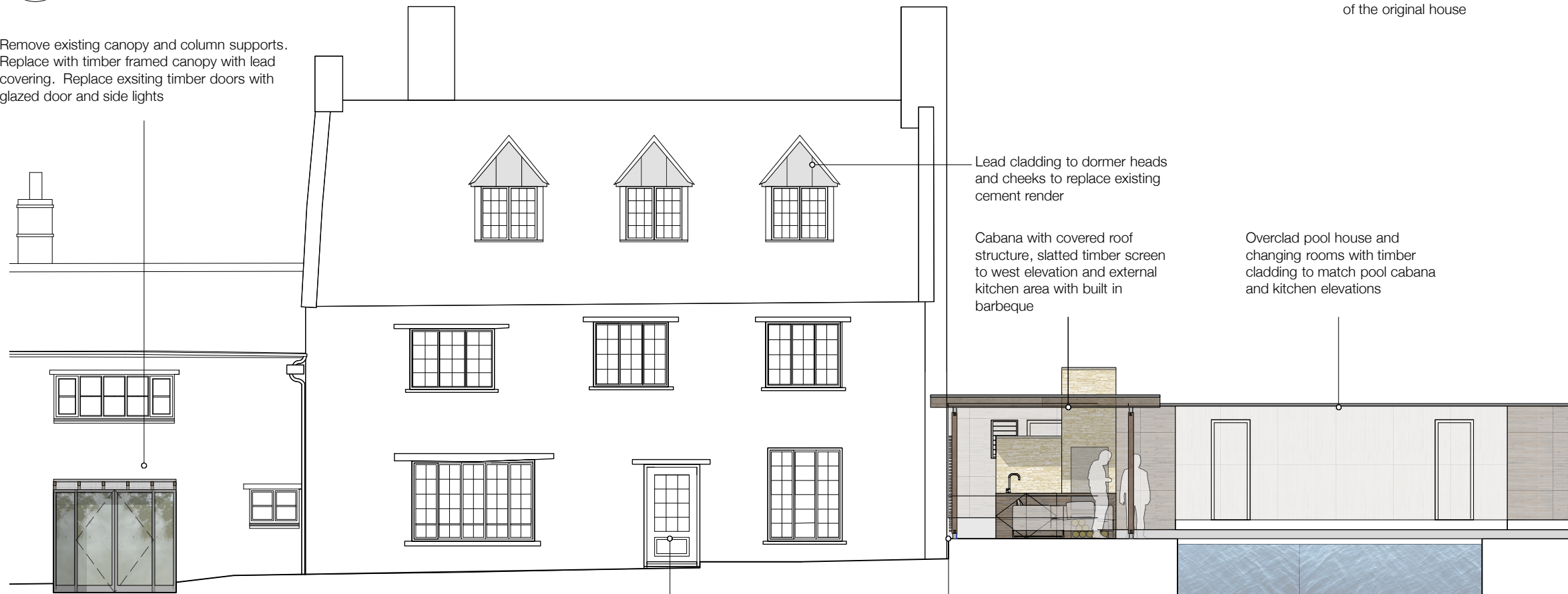
1 Proposed South Elevation - Part 1 Scale: 1:100
