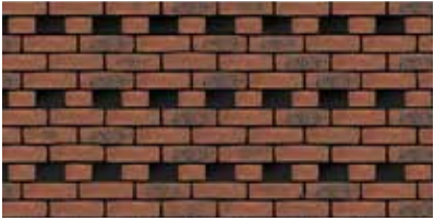
Perforated brick pattern with removed headers
