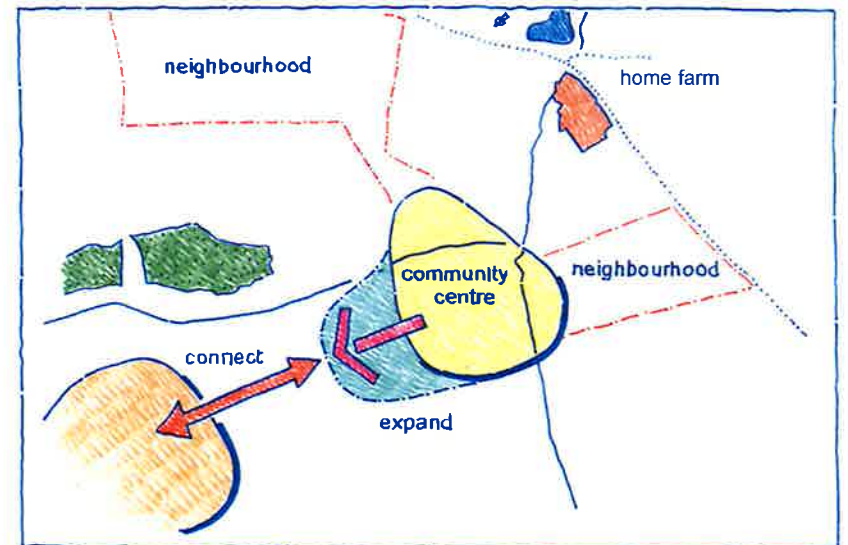
Place the centre so that it can grow in later phases and link with other community centres.
