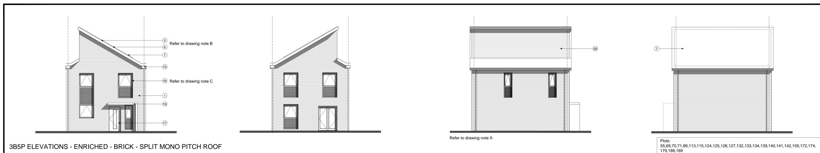
Note: Handed Enriched plots should maintain a south facing roof for PV requirements
