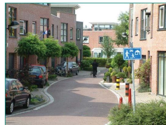
Meandering road providing traffic calming
