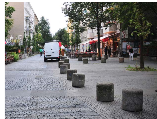
Bollards to demarcate vehicular and pedestrian zone
