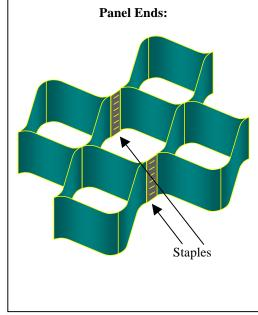
Below are illustrations of the correct stapling procedure for joining both edges and ends of panels together;
