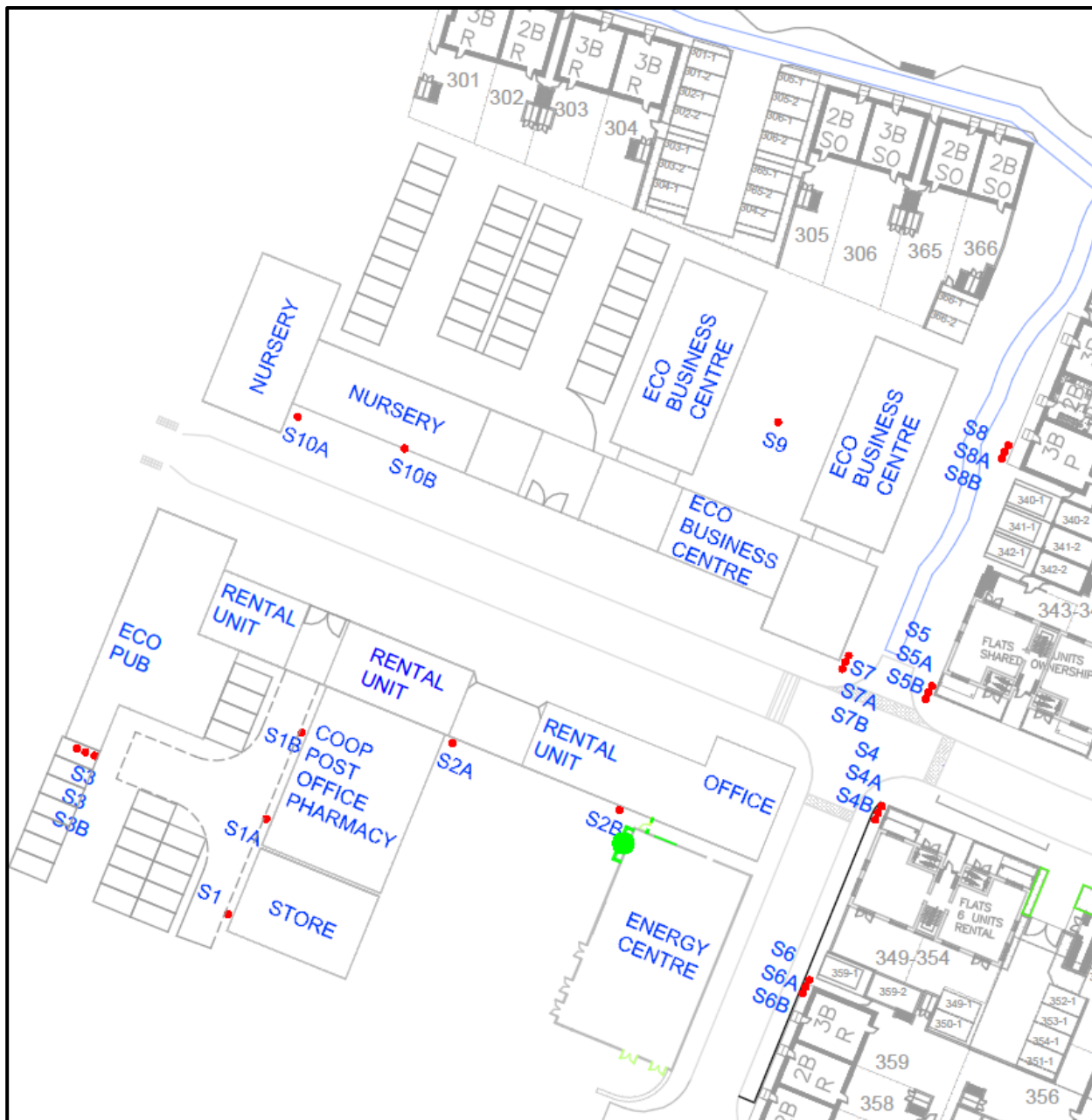
Figure 1: Study area showing buildings included in the dispersion modelling for the Bicester Energy Centre and discrete receptors identified as solid red circles. The Energy Centre stack is shown in green.
