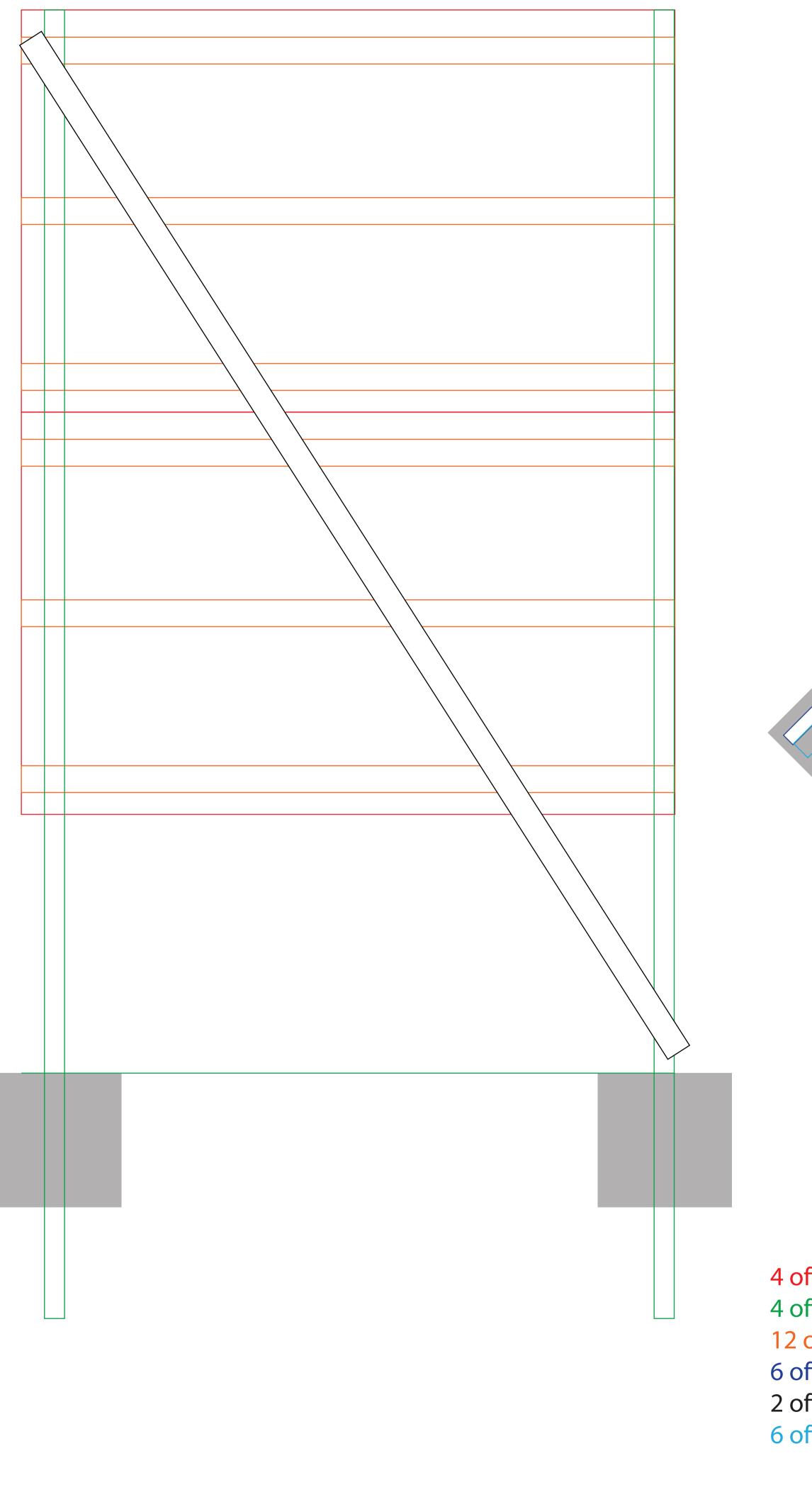
4 off 3mm dibond panels (1.5m x 2.44m) 4 off 4.88m 150mm x 75mm timber uprights 12 off 2.44m 100mm x 50mm timber crossrails 6 off 2.446m 100mm x 50mm timber front/back stays 2 off 4.88m 100mm x 50mm timber 'z' braces 6 off .75m 100mm x 75mm timber pointers
