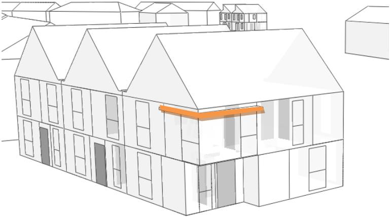
Figure 7. 3D image of Plot 281 with the overhang added on the bay window
