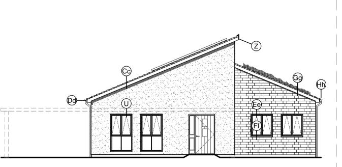
TYPE - 8 WALLS - ½ Bekstone; ½ Render ROOF - Sawtooth - [slate + green] Front Elevation indicated, refer to Section 96a Dwgs AA2699(2) 2118 & 2122
