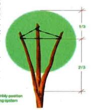
In the case of a loadbracing system, the height is not as important as ensuring that the cables are as vertical as possible.
