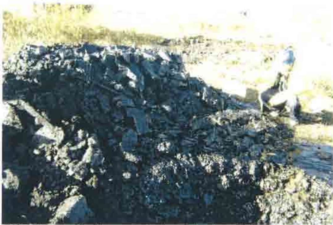
TP06 – Example of coal tar contamination and abundant rubble
