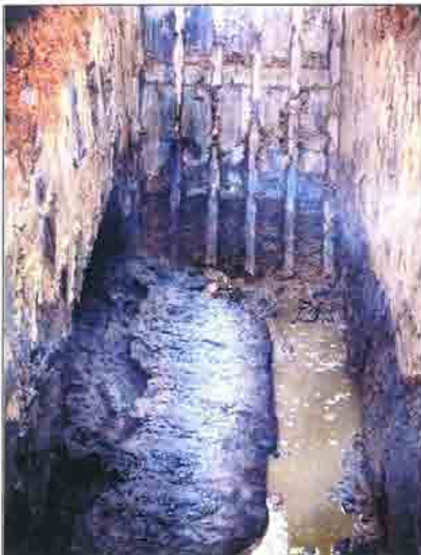
Plate 2: South eastern face of trial pit - significant contamination of alluvium (strong gas works odour)
