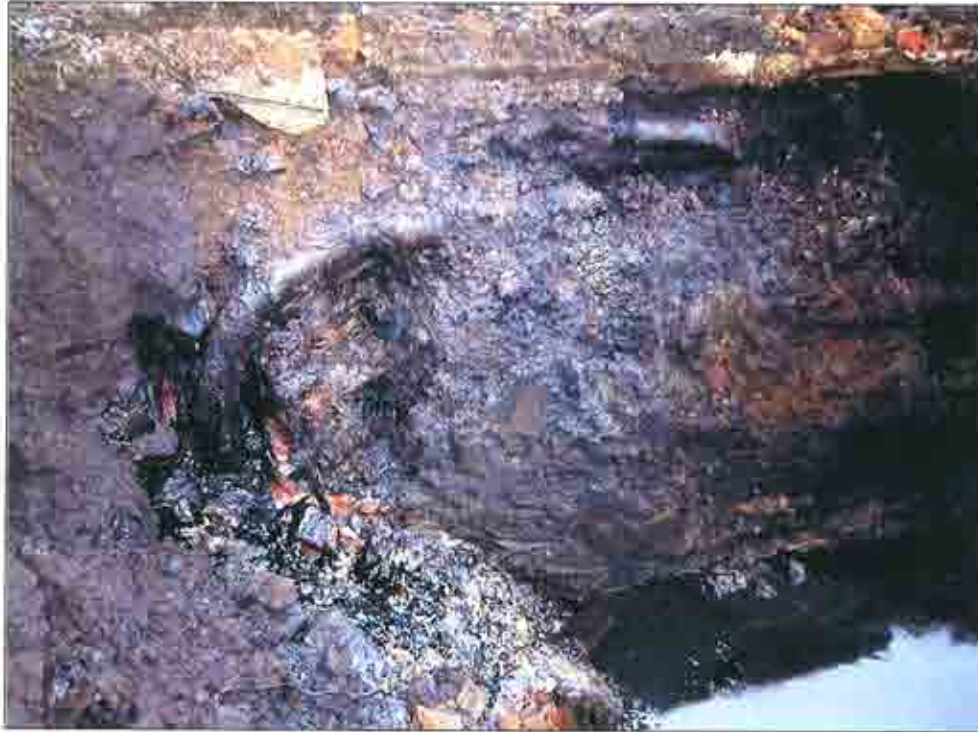
Plate 15: Significant influx of tarry residues on the northwestern face of the trial pit
