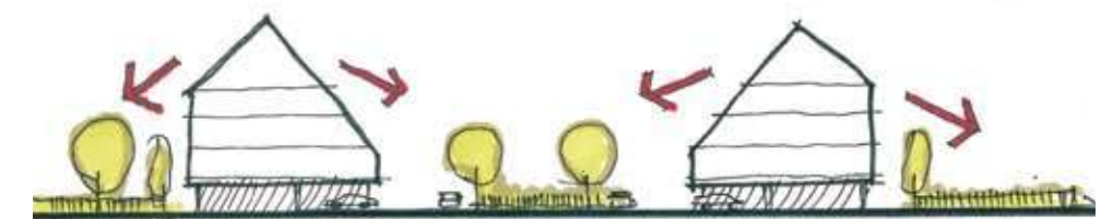
Roof forms designed to allow maximum views from all balconies into the amenity space whilst preventing overlooking into the balconies below
