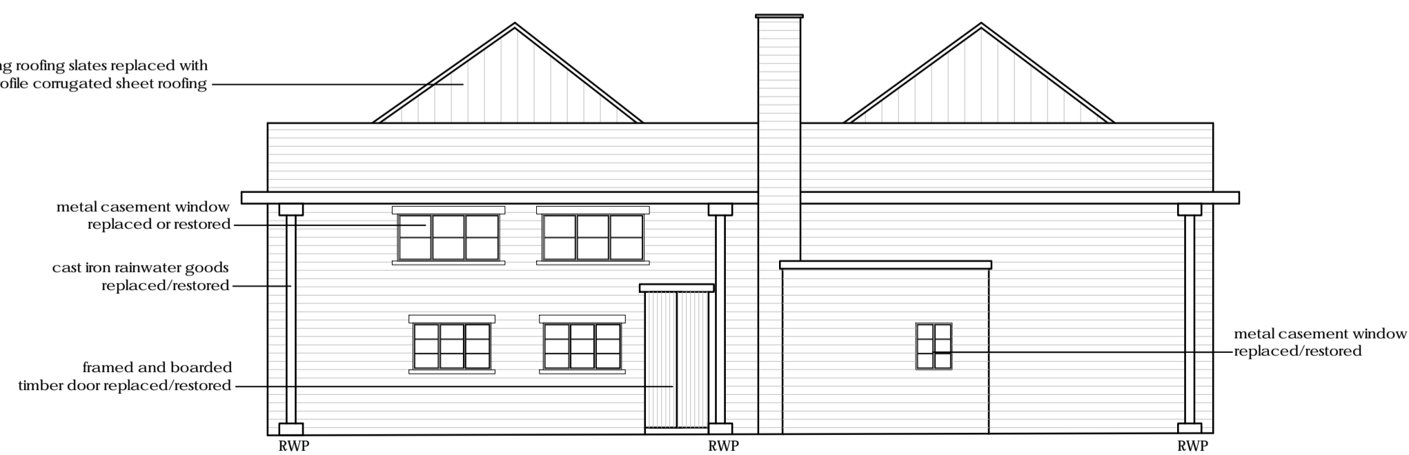
BUILDING 119 SOUTH ELEVATION - PROPOSED
