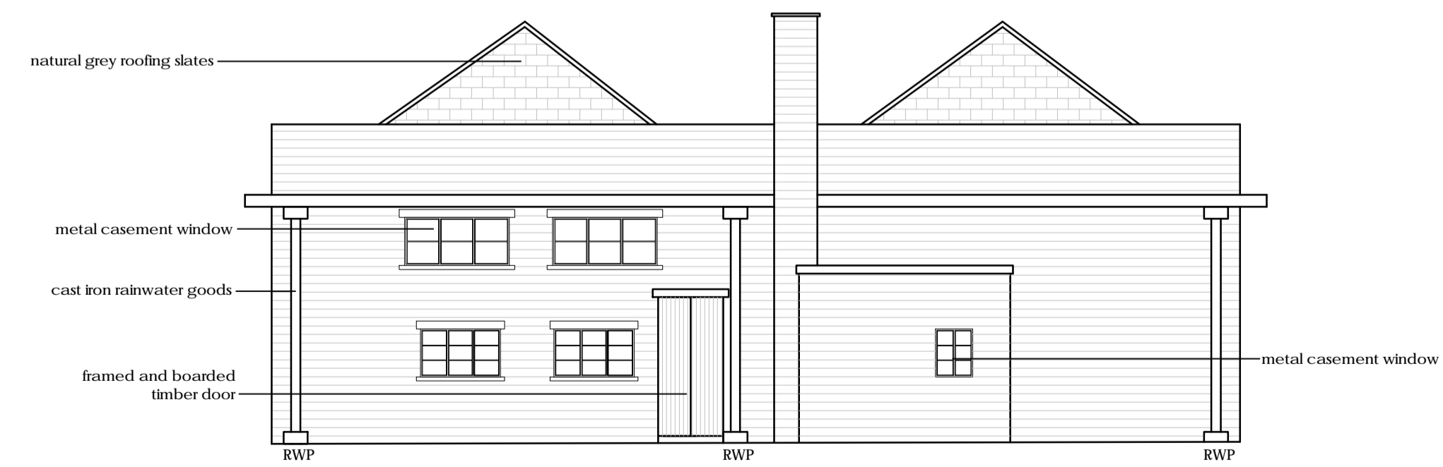
BUILDING 119 SOUTH ELEVATION - EXISTING
